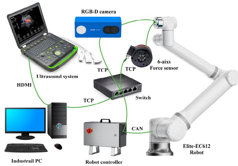
**Figure 14.** Hardware architecture of experimental setup.
