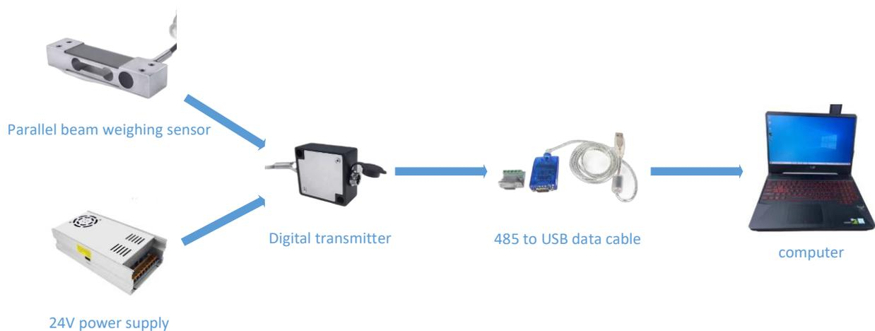
**Figure 7.** Schematic diagram of load cell experiments.
