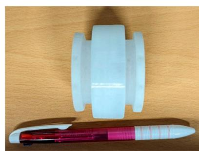
**Figure 5.** Printed membrane resonator.
