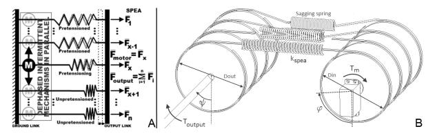
When all the springs are in the unpretensioned phase (and thus, all the input drums at the equilibrium position), a positive  $\psi_{\text{output}}$  will extend all the parallel springs and, as such, generate a negative  $T_{\text{output}}$ . In contrast, for a positive  $\psi_{\text{output}}$ , all the springs will sag and the  $T_{\text{output}}$  is 0 Nm.
