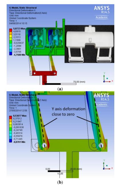
To achieve a fast pneumatic AM, the actuator is necessary to reduce the volume of the chamber. Small chambers have small motion and to use them as actuators for grippers is necessary a mechanism to achieve enough motion of the fingers. Figure 9 has two small AM pneumatic actuators with only one lobe. Every finger is moved by one pneumatic AM actuator. The fingers are rigid and they are joined to the gripper and chassis with two shafts per finger (shafts in Figure 9a). An equivalent gripper
