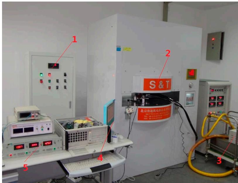
**Figure 2.** Experimental setup: (1) power; (2) loading device; (3) power supply for temperature loading system; (4) computer with data acquisition card, which collects input magnetic field intensity  $H$  and output magnetic induction intensity  $B$ ; and (5) control device for magnetic field.
