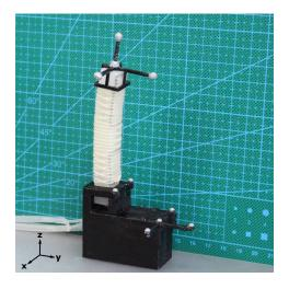
**Figure 4.** Motion capture marker setup for trajectory measurements. The two center markers on the tip of the actuator formed its tip vector. Other markers were used as a reference.
