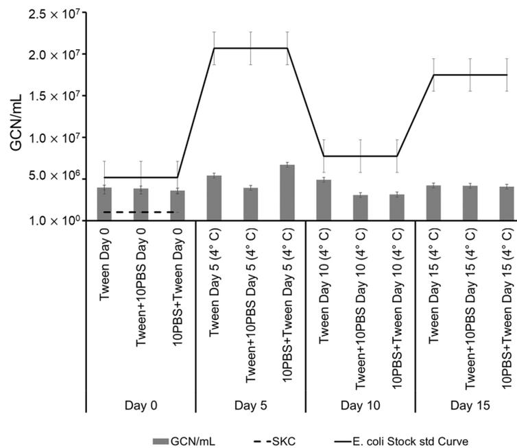
**Figure 3.** Real-time PCR analysis of the *E. coli* samples archived for 15 days at 4 °C collected in Tween, amended with 10% PBS (Tween + 10PBS) or being added to 10% PBS (10PBS + Tween). The GCN/mL values for the samples collected on Day 0 with the SKC impinger are indicated with a dashed line. The solid line represents the non-aerosolized *E. coli* stock.
