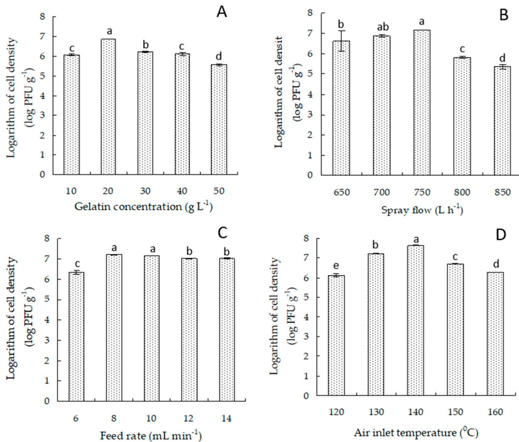
**Figure 1.** Effects of gelatin concentration (A), spray flow (B), feed rate (C), and air inlet temperature (D) on cell density of *Bdellovibrio* sp. strain F16 in the spray-dried powder. Data presented as the mean of triplicate spray-drying trials and standard deviations (SD) are indicated by the vertical bars. Bars with different lowercase letters are statistically different ( $p < 0.05$ ).
