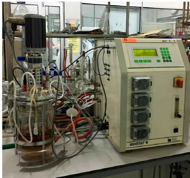
**Figure 1.** The photograph of 2 L stirred tank bioreactor setting (BIOSTAT, B. Braun Biotech International, Germany) for BLIS production by *L. lactis* Gh1.
