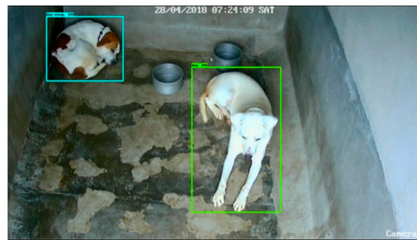
Figure 1. Detection of dogs by the BlyzerDS system using a neural network. Different colours in the bounding boxes show the system correctly scoring two individuals (blue = asleep; green = awake).
