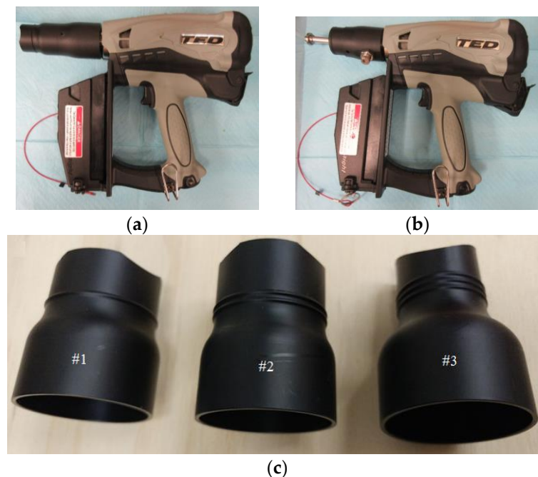
Figure 2. The non-penetrating captive bolt device (Turkey Euthanasia Device). (a) Device with adapter 1; (b) Device with adapter removed and bolt head exposed; (c) Subject adapters [36].
