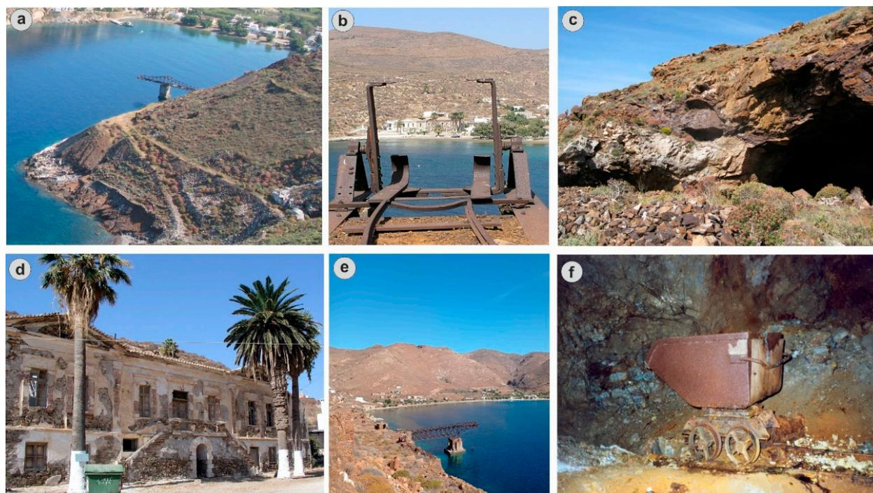
**Figure 11.** Field and underground photos showing evidence of mining activity at Serifos. (a,b) Loading bridges at Megalo Livadi; (c) entrance of gallery at Megalo Livadi; (d) the headquarters of the iron ore mines at Megalo Livadi; (e) loading bridge at Koutalas; (f) mining wagon in a Koutalas mine.
