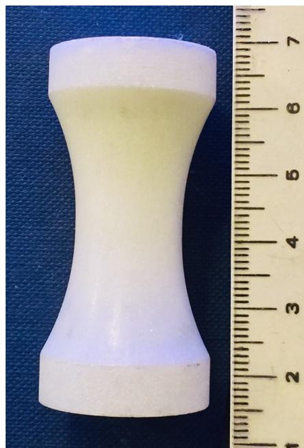
**Figure 1.** Geometrical form of the sample of Carrara marble deformed in axial compression for this study (cm scale).
