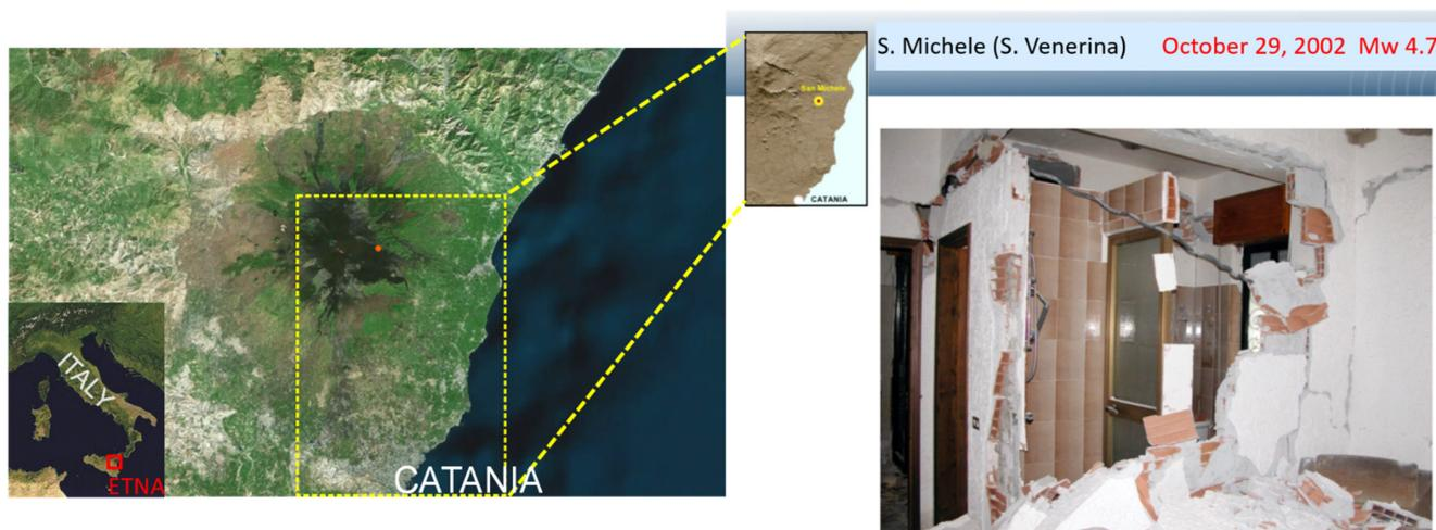
**Figure 1.** Map of Etna (Italy) and an example of non-structural damage inside a reinforced concrete building due to an Mw 4.7 earthquake in October 2002 (modified from Azzaro et al. [15]).
