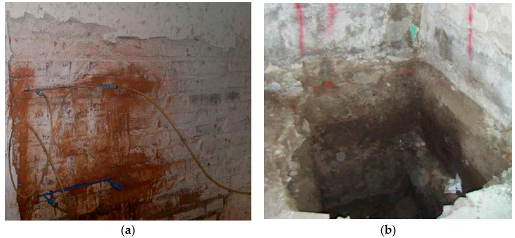
Figure 4. (a) Double flat jack test performed on the masonry walls; (b) foundation inspection pit.
