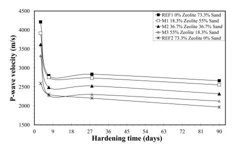
Figure 1. Variation of P-wave velocity vs. days of hardening.
