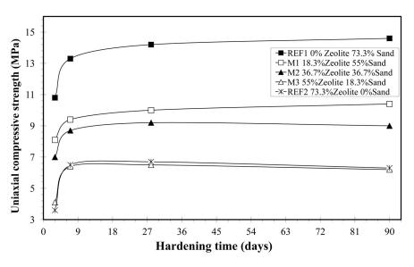
Figure 3. Variation of uniaxial compressive strength vs. hardening time.
