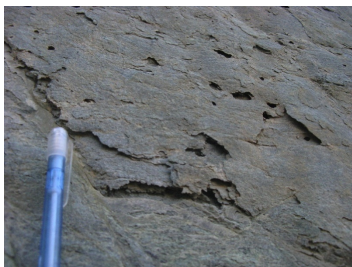
Figure 5. Scaling in serpentinites at the La Carrasca quarry front. In this case, the exposure faces north, where marked changes in temperature and insulation take place.
