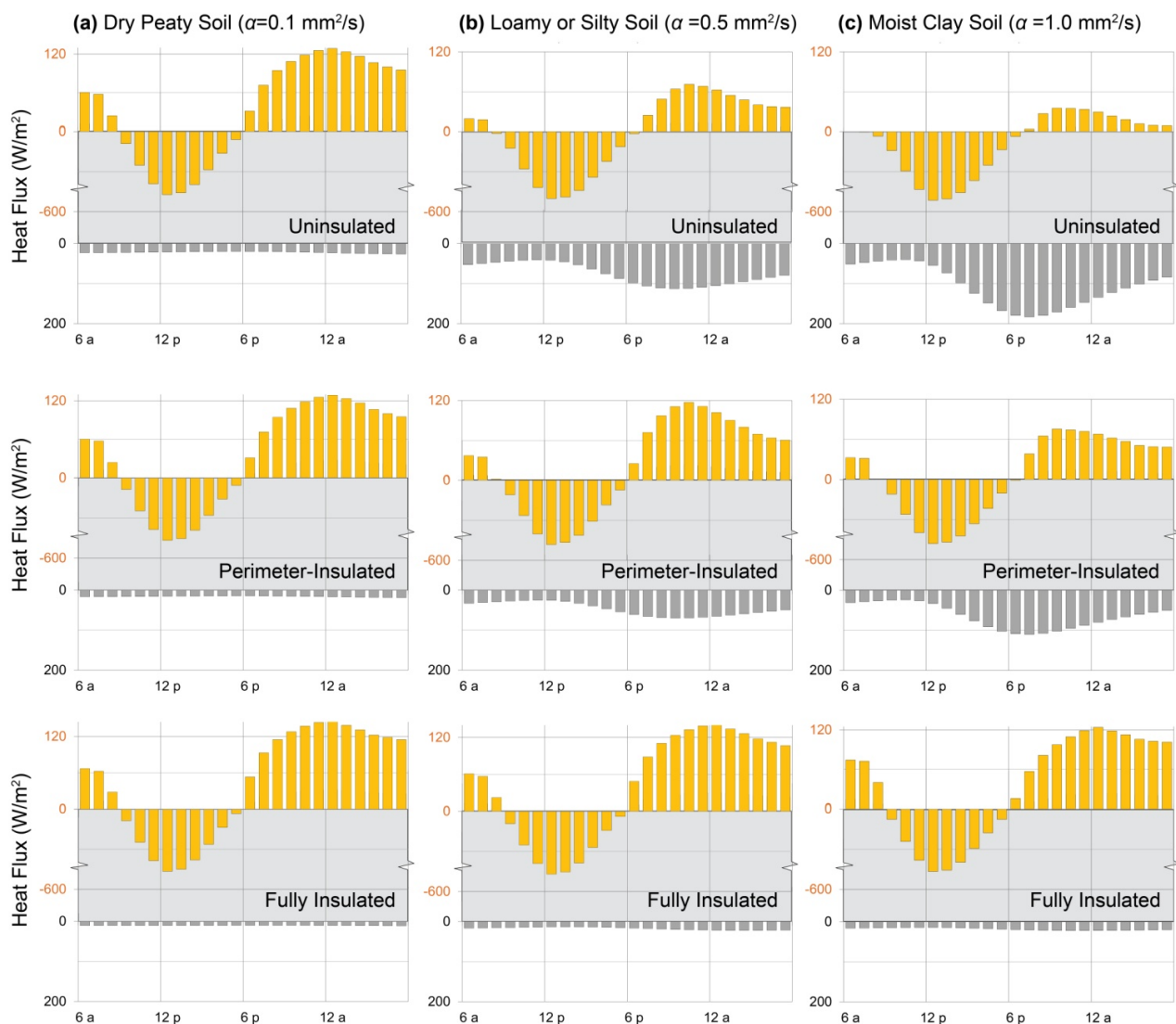
Figure 9. Direct gain mass floor. Heat fluxes across indoor (upper) and ground (lower) surfaces of 10 cm (4 in.) concrete slabs-on-grade over soils with thermal diffusivities of (a) 0.1 \text{ mm}^2/\text{s} , representative of a dry peaty soil; (b) 0.5 \text{ mm}^2/\text{s} , representative of many silty and loamy soils; and (c) 1.0 \text{ mm}^2/\text{s} , representative of a moist clay soil. The top row illustrates patterns characteristic of uninsulated slabs; the middle row adds perimeter R-10 insulation, and the bottom row employs full under-slab R-10 insulation. All models were simulated on a typical sunny January day in Denver, Colorado. Patterns show the strong influence of soil thermal properties on floor thermal storage performance, particularly when the solar collection surface lies on moist or fine-grained soils.
