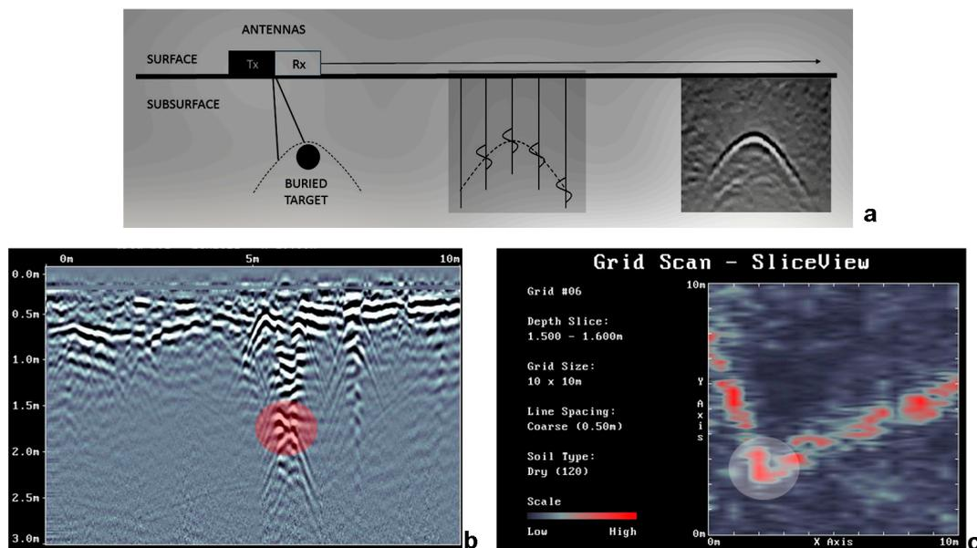
**Figure 3.** The upper image shows geometry of the most common mode of GPR data acquisition, referred to as “reflection mode” coverage. In (a), single transmitter (Tx) and receiver (Rx) antennae are transported over the ground surface in a fixed configuration above a buried target, resulting in hyperbolic time-distance behavior. The lower images show, in (b), a typical radargram (B-scan or GPR section). In (c), the relative depth map (C-scan or GPR depth-slice).
