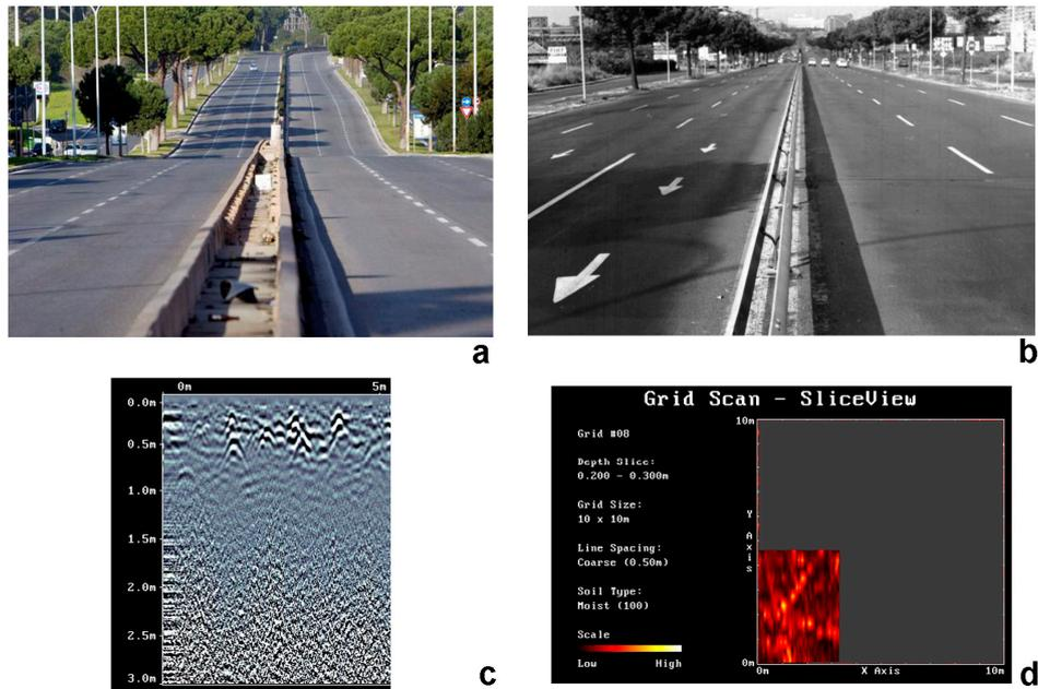
**Figure 6.** The upper images show Via Cristoforo Colombo in recent times (a) and during the 1950s (b). The lower images clearly show the very shallow root architecture of the pine trees beneath the asphalt road surface (hyperbolic events in (c) and yellow elongated anomalies in (d)). Note, however, that the asphalt surface is not yet damaged by root growth.
