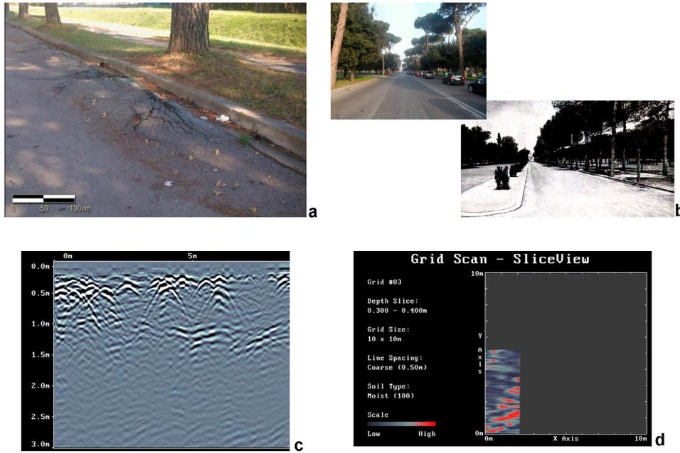
**Figure 5.** In (a), damaged asphalt along Viale delle Terme di Caracalla is shown. This tree-lined street was constructed in 1940s, as shown in (b). Strong hyperbolic events and red elongated anomalies in the first 0.4 m, observed on both the radargram (c) and depth map (d) image the root architecture beneath the asphalt.
