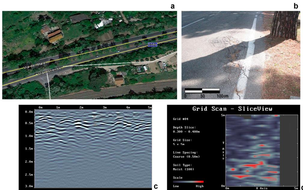
**Figure 4.** This figure shows the area of investigation along the SS8bis (a), with damage to asphalt due to the pine root growth and pavement uplifting (b). Several hyperbolic events and red elongated anomalies within the first 0.4 m on both the radargram (c) and depth slice map (d) are due to the root architecture beneath the asphalt.
