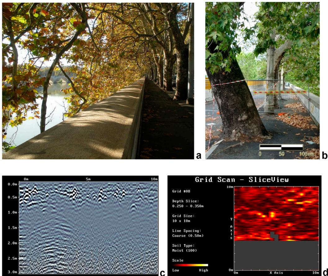
**Figure 7.** The upper images illustrate the critical situation of the plane trees between the embankments of the Tiber River and Lungotevere Street (a,b). The lower images illustrate the GPR results collected around the leaning tree (c,d) and highlight critical conditions in the first 0.3 m beneath the pavement. Note that the grey area in (d) represents the area with no GPR data parallel to the embankment.
