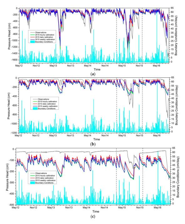
**Figure 5.** Pressure head values modeled for the period from May 2012 to September 2016. The model is calibrated using hourly, daily, and weekly data for the period from April to December 2015 (limited by vertical straight lines in the picture): pressure head values at depths of 42 cm (**a**), 71 cm (**b**), and 116 cm (**c**).
