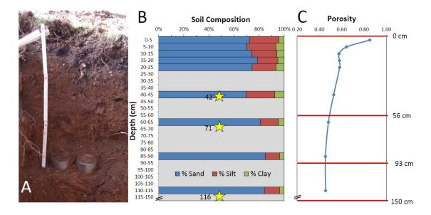
**Figure 2.** (**A**) Undisturbed soil cylinder samplers. (**B**) Soil composition profile; yellow stars correspond to sampling points and (**C**) porosity profile obtained through laboratory analysis of the field samples. These values are used for the ROSETTA pedotransfer function. The red lines in (**C**) represent the interfaces between the three layers of the adopted soil model.
