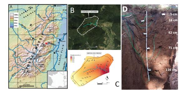
**Figure 1.** (**A**) Regional map of the Vosges Massif and location of the Strengbach catchment. (**B**) Contour map of the Strengbach watershed. (**C**) Topographic map of the Strengbach watershed and location of the studied weathering profile (map from OHGE). (**D**) Vertical profile in the experimental spruce parcel (blue star in Figure 1C) where sensors have been installed.
