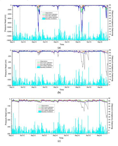
**Figure 4.** Pressure head values modeled for the period from May 2012 to September 2016. The model is calibrated using hourly, daily, and weekly data for the period from June to September 2012 (limited by vertical straight lines): pressure head values at depths of 42 cm (**a**), 71 cm (**b**) and 116 cm (**c**).
