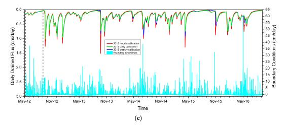
**Figure 6.** Modeled cumulative (**a**) and daily (**b** and **c**) drained flux at the depth of 150 cm for the period from May 2012 to September 2016. The model is calibrated using hourly, daily, and weekly data for the periods from April to December 2015 (**b**) and from June to September 2012 (**c**) (calibration period is limited by vertical straight lines on each picture).
