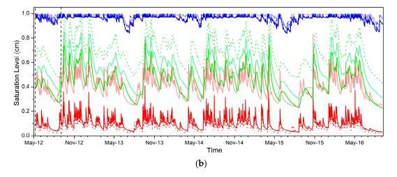
**Figure 7.** Saturation level modeled for the period from May 2012 to September 2016 for a three-layer model. The model is calibrated using hourly, daily and weekly data for the periods from April to December 2015 (**a**) and from June to September 2012 (**b**) (calibration period is limited by vertical straight lines on each picture).
