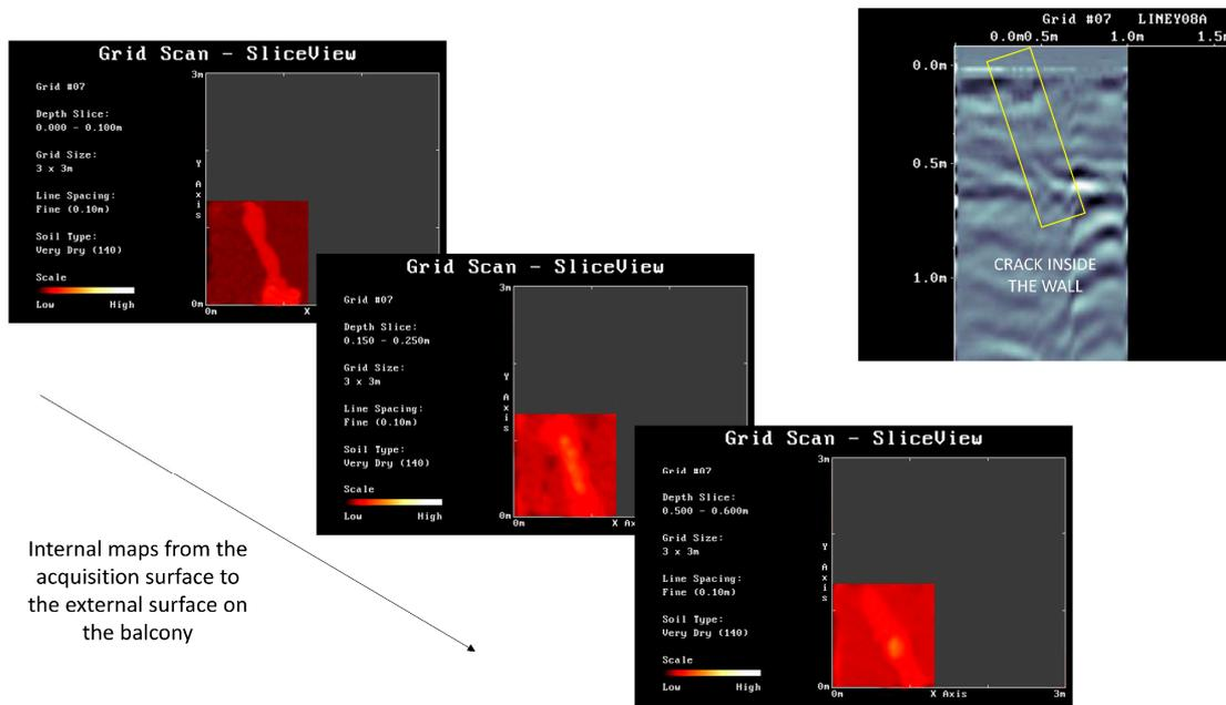
**Figure 7.** Both the GPR profiles (top right) and the three depth-slices show the presence of the crack and its inner geometry passing through the 0.5 m thick masonry from side to side.
