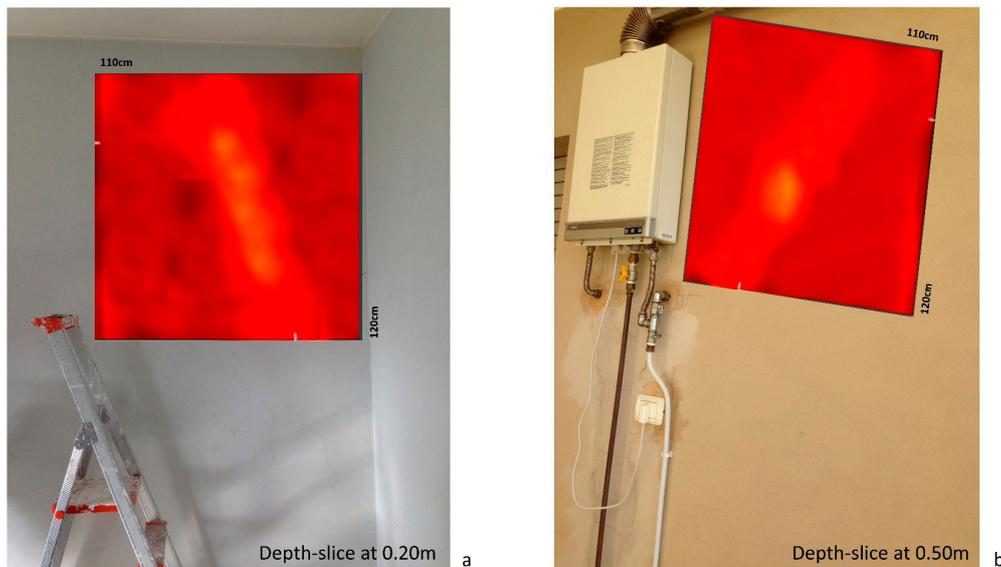
**Figure 8.** (a) The depth-slice at 0.2 m inside the masonry, revealing its inner geometry; (b) The depth-slice at 0.5 m of the same crack in the wall from the balcony.
