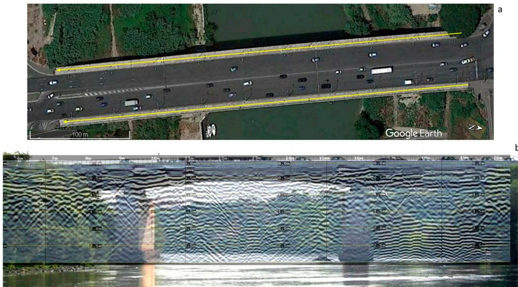
**Figure 9.** (a) The orientation of the profiles acquired along the two “wings” of the Marconi Bridge (Google Earth image); (b) is an overlap attempted to show a GPR profile showing the thickness of the “wings” and the penetration of the radar signal through the pylons and up to the surface of the river water below.
