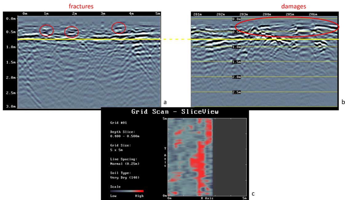
**Figure 11.** (a) Illustrates the internal damage to the “winged” structure of the bridge; (b) Shows superficial damage linked to the failure of the travertine surface of the sidewalks; (c) highlights the depth-slices showing evident anomalies due to detachments and cracks (in red).
