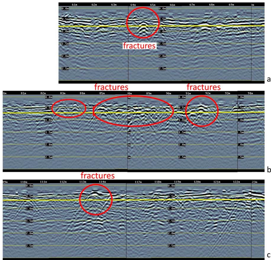
**Figure 10.** (a–c) show in greater detail the most obvious anomalies found close to the visible damaged part of the bridge (Figure 6). The yellow portion clearly shows the thickness of the wings at about 0.6 m.
