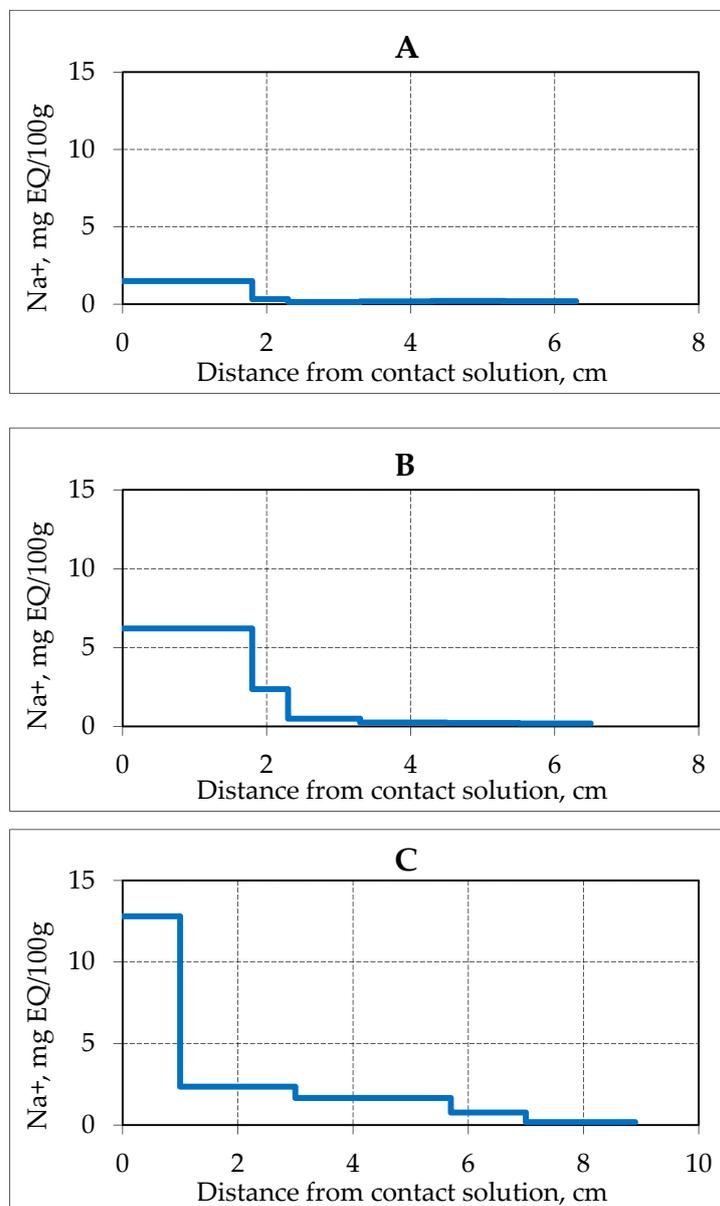
**Figure 8.** Accumulation of  $\text{Na}^+$  ions in samples of frozen hydrate saturated sand (sand 2,  $W = 16\%$ ) after 3 h of contact with NaCl solution of various concentrations at a temperature of  $-3\text{ }^{\circ}\text{C}$ . (A–C)—solution concentration, respectively, 0.1, 0.2 and 0.4 N.
