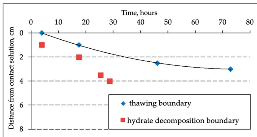
**Figure 4.** Experimental assessment of the gas hydrate decomposition front in porous media and the thawing front in frozen hydrate-containing sandy samples (sand-1,  $W = 14\%$ ) when interacting with 0.2 N NaCl salt solution at the temperature  $-4\text{ }^{\circ}\text{C}$ .
