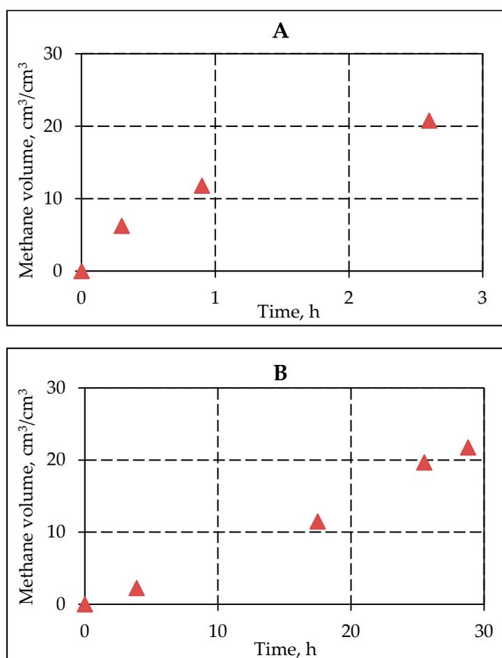
**Figure 10.** Methane emission in frozen hydrate saturated samples of sand (sand 1) during the gas hydrate dissociation in the pore space as a result of interaction with 0.2 N NaCl salt solution at temperatures  $-2.5\text{ }^{\circ}\text{C}$  (A) and  $-4\text{ }^{\circ}\text{C}$  (B).
