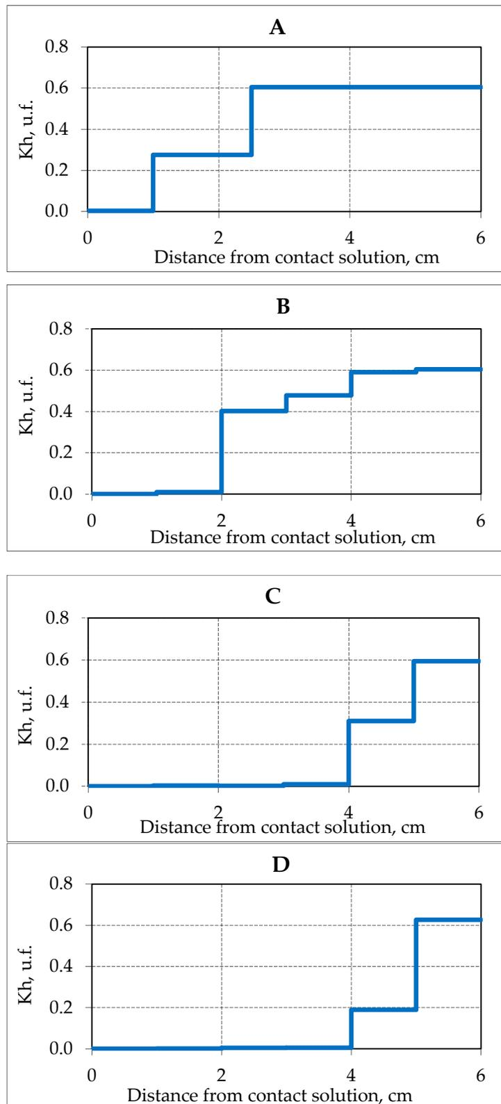
**Figure 3.** The change in the hydration coefficient ( $K_h$ ) in frozen hydrate saturated samples of sand (sand 1,  $W = 14\%$ ) in time when interacting with 0.2 N NaCl salt solution at a temperature of  $-4\text{ }^\circ\text{C}$ . (A–D) is the time of interaction with the salt solution, respectively, 3.9, 17.5, 25.5 and 28.8 h.
