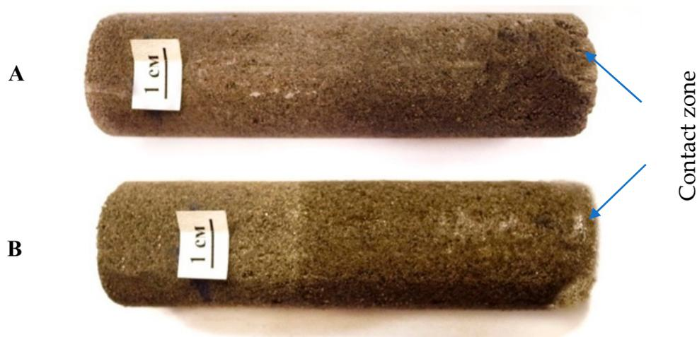
**Figure 5.** Frozen sandy samples (sand 2,  $W = 15\%$ ) before (A) and after interaction (B) with 0.2 N NaCl solution at  $-3\text{ }^{\circ}\text{C}$ .
