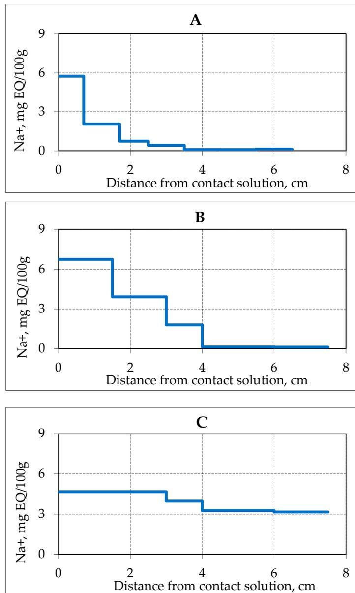
**Figure 6.** Accumulation of Na<sup>+</sup> ions in samples of frozen hydrate saturated sand (sand 2, W = 16%) over time when interacting with 0.2 N NaCl solution at a temperature −2.5 °C. (A–C)—the time of interaction with salt solution, respectively, 0.3, 0.9 and 2.6 h.
