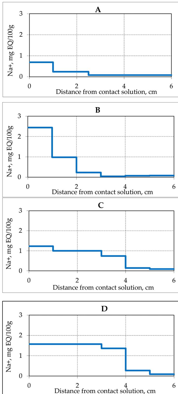
**Figure 2.** Accumulation of Na<sup>+</sup> ions in samples of frozen hydrate saturated sand (sand 1, W = 14%) in time when interacting with 0.2 N NaCl solution at a temperature of -4 °C. (A–D) is the time of interaction with the salt solution, respectively, 3.9, 17.5, 25.5 and 28.8 h.
