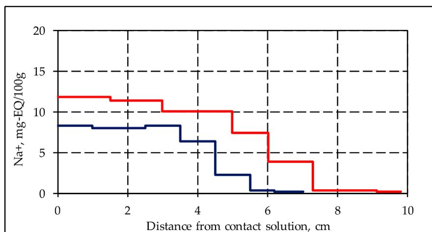
**Figure 1.** Salt ion accumulations ( $\text{Na}^+$ ) in frozen sand samples (sand 1,  $W = 14\%$ ) containing (red line) and not containing (blue line) hydrate in porous media after 46 h of contact with 0.2N NaCl solution under the temperature  $-4\text{ }^\circ\text{C}$ .
