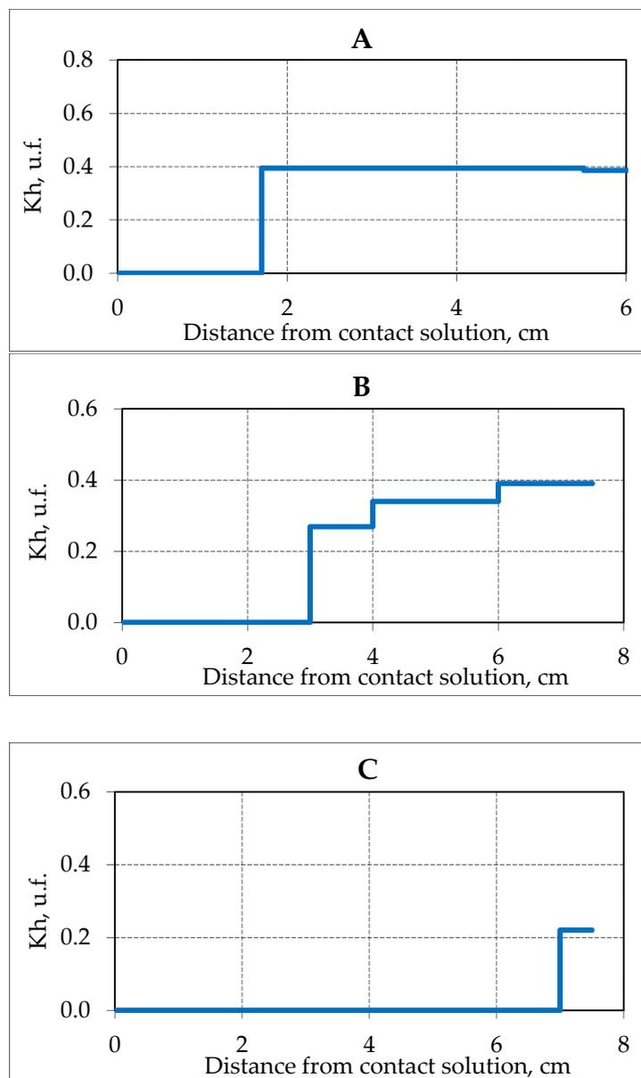
**Figure 7.** The change in the hydration coefficient ( $K_h$ ) in samples of frozen hydrate saturated sand (sand 2,  $W = 16\%$ ) in time when interacting with 0.2 N NaCl solution at a temperature of  $-2.5\text{ }^{\circ}\text{C}$ . (A–C) is the time of interaction with the salt solution, respectively, 0.3; 0.9; 2.6 h.
