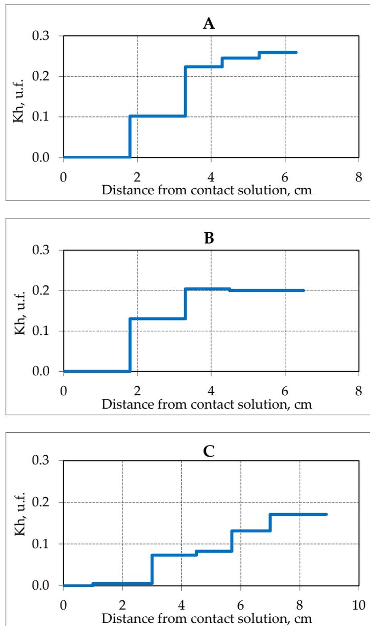
**Figure 9.** Changes in the hydration coefficient ( $K_h$ ) in samples of frozen hydrate saturated sand (sand 2,  $W = 16\%$ ) after 3 h of contact with NaCl solution of various concentrations at a temperature of  $-3\text{ }^\circ\text{C}$ . (A–C) solution concentration, respectively, 0.1, 0.2 and 0.4 N.
