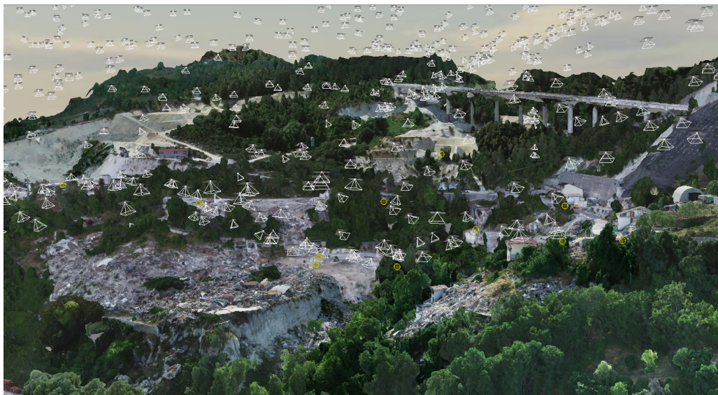
Figure 11. Optimized mission plan: camera locations and angles represented as triangular prisms.
