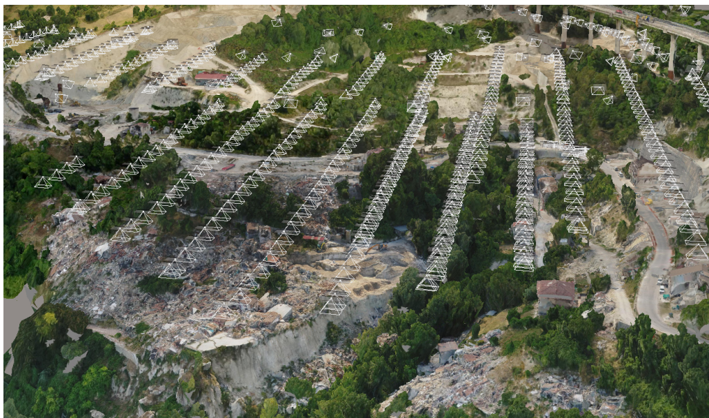
Figure 10. Industry standard mission plan: camera locations and angles represented as triangular prisms.
