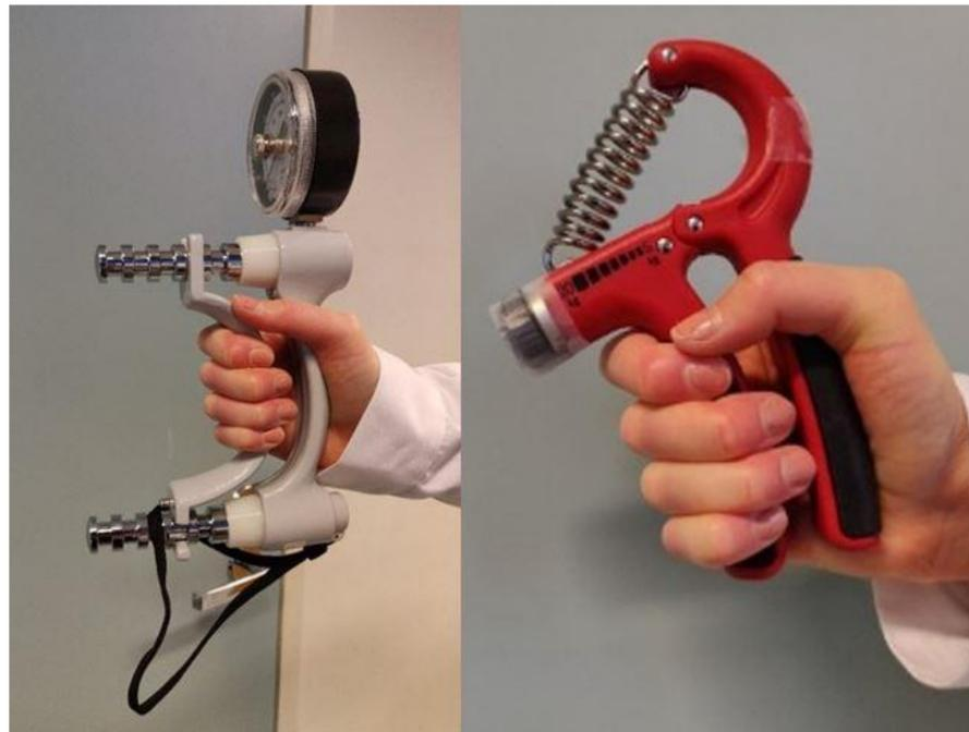
**Figure 1.** Hand grip strength measurement device (left) and hand grip endurance task device (right).
