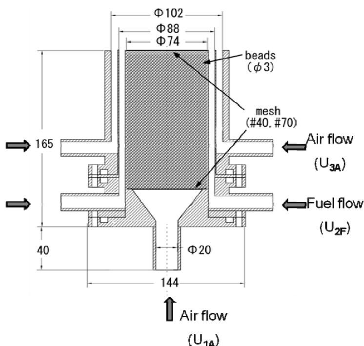
So far, we have examined the flame structure and emission characteristics of soot and  $\text{NO}_x$  in the triple port burner [5]. Compared with a so-called co-axial burner, the contact area between fuel and air is larger due to the center air injection, which enables the promotion of both substances' admixture and reaction [8,9]. In the triple port burner, there are two flames, inner and outer flames, which could reduce PAH and soot formations largely.
