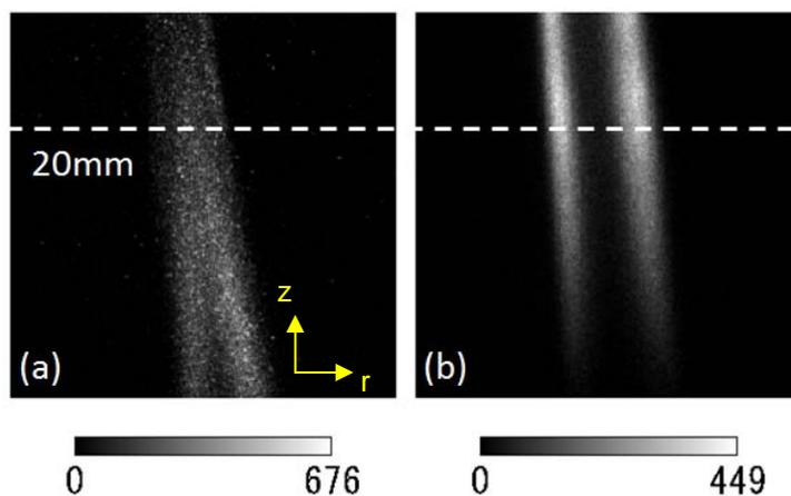
**Figure 6.** Profiles of PAH-LIF and LII signals in the triple port burner at  $z = 20\text{mm}$ .
