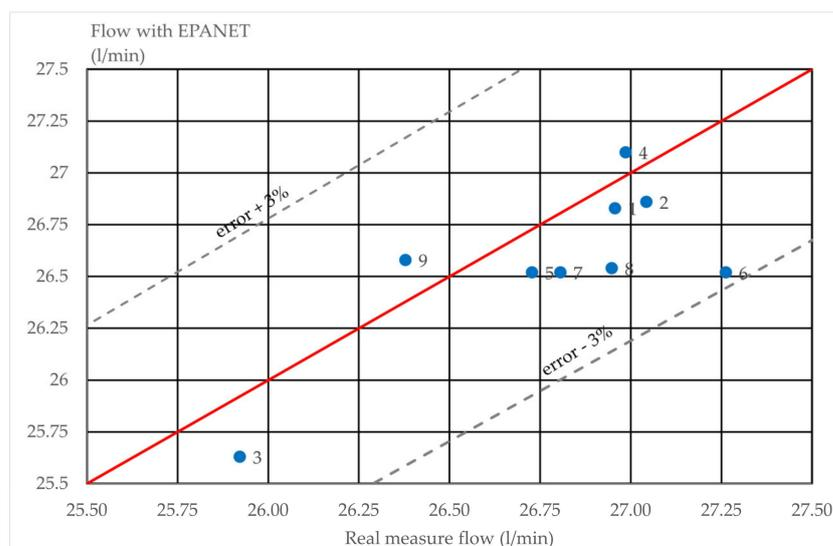
**Figure 3.** Real flow measure vs. EPANET flow for each series of measurements. In this figure, each blue circle corresponds to a test in Table 2.
