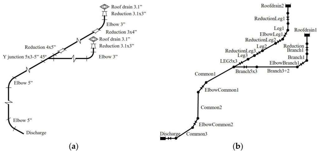
Figure 4. (a) SRDS model in SIPHONITEC®. (b) SRDS model in EPANET.
