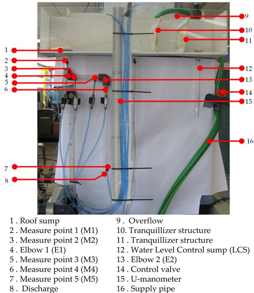
**Figure 1.** Laboratory SRDS small-size test model.
