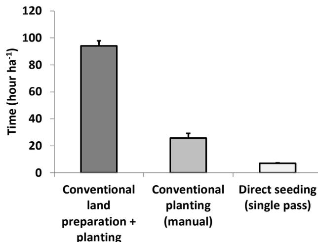
**Figure 1.** Comparison of the average time required for conventional land preparation and conventional planting of maize (land preparation using an animal drawn *maresha* and planting by hand), for conventional planting of maize only (following conventional land preparation), and for direct seeding of maize using a 2BFT-100 seeder powered by a 15 HP two-wheel tractor in an untilled land in Hawassa Ethiopia (source: [23]).
