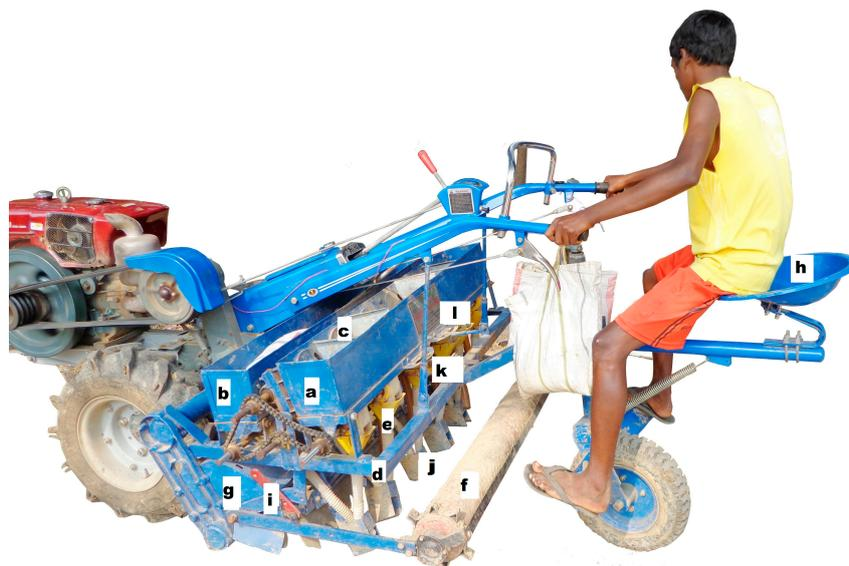
**Figure 1.** A Versatile Strip Seed Drill (VSSD) attached with Dongfeng-type 2-wheel tractor. Parts specification: (a) = seed box; (b) = fertilizer box; (c) = vertical disk seed meter; (d) = toolbar frame; (e) = seed delivery tube; (f) = pressing roller; (g) = cover of rotary shaft and tines; (h) = driving seat for transportation; (i) = depth control bar; (j) = furrow opener; (k) = seed and fertilizer off/on lever; (l) = seed rate adjustable lever for fluted roller type seed meters.
