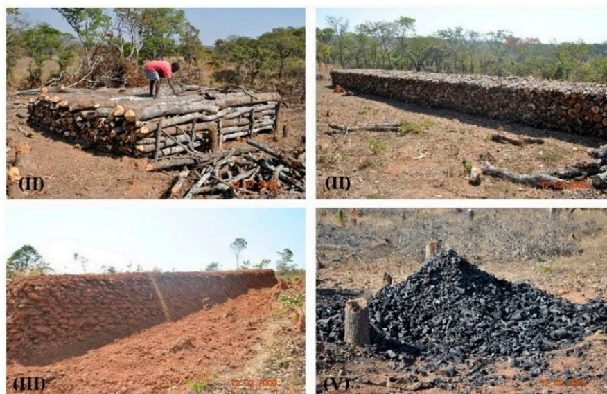
**Figure 2.** Processes of charcoal production by traditional earth kiln. Upper images (II) show the process of log piling into clamp, and the lower left image (III) shows covering of the clamp with dung and soil lumps, while the lower right image (V) shows the harvesting of charcoal and packaging it into bags. The steps number (I,IV) are not represented in this figure.
