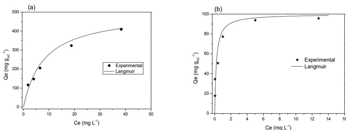
**Figure 3.** Equilibrium adsorption isotherms of CB (a) and 2,4-D (b) over activated carbon ( $35 \text{ }^\circ\text{C}$ ). Symbols represent experimental data and lines are fitting to the Langmuir equation.
