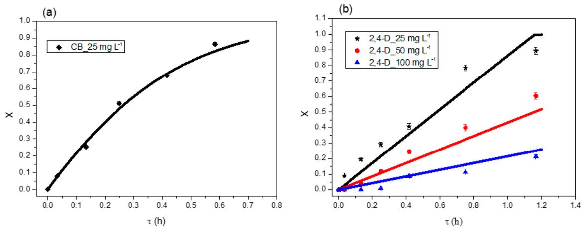
**Figure 6.** Kinetic modelling of CB (a) and 2,4-D (b) biodegradation in USPBRs. Lines represent fitting to the Michaelis-Menten model (T = 35 °C).
