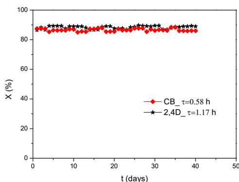
**Figure 5.** Stability of the USPBR system during long operation periods. ( $[\text{CB}]_{\text{in}}$  or  $[\text{2,4-D}]_{\text{in}} = 25 \text{ mg L}^{-1}$ ,  $T = 35 \text{ }^{\circ}\text{C}$ ).
