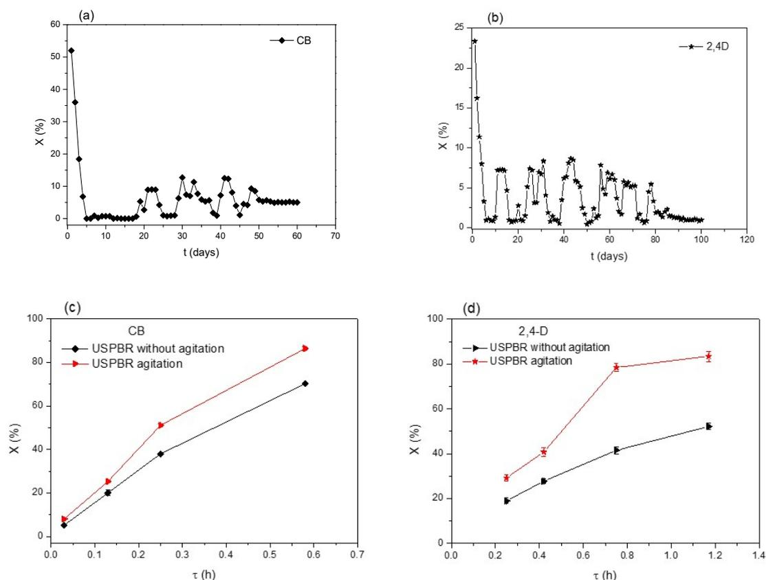
**Figure 4.** (a,b) Acclimatization and stabilization period of USPBRs for CB ([CB]<sub>in</sub> = 25 mg L<sup>-1</sup>, T = 35 °C,  $\tau$  = 0.033 h) and 2,4-D ([2,4-D]<sub>in</sub> = 100 mg L<sup>-1</sup>, T = 35 °C,  $\tau$  = 0.033 h). (c,d) Performance of USPBRs at different space times for CB and 2,4D ([CB]<sub>in</sub> or [2,4-D]<sub>in</sub> = 25 mg L<sup>-1</sup>, T = 35 °C), with and without stirring.
