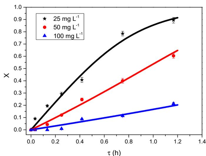
**Figure 7.** Fitting to the Michaelis-Menten model, including substrate inhibition, during 2,4-D biodegradation in USPBR. Continuous lines represent the fitting to the extended Michaelis-Menten.
