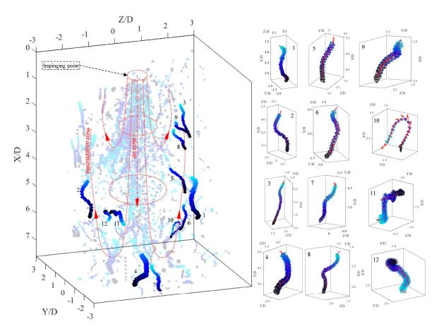
**Figure 5.** Sequence of air bubbles entrained by the vertical plunging jet and reconstructed by means of the volumetric shadowgraph technique. The plunging jet is downward from the top, with X/D = 0 indicating the water surface.
