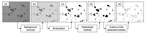
Figure 4. Steps for the boundary detection: original image (a); image after background removal (b); binary image (c); image after watershed operation (d); final image containing the outline of the detected air bubbles (e).
