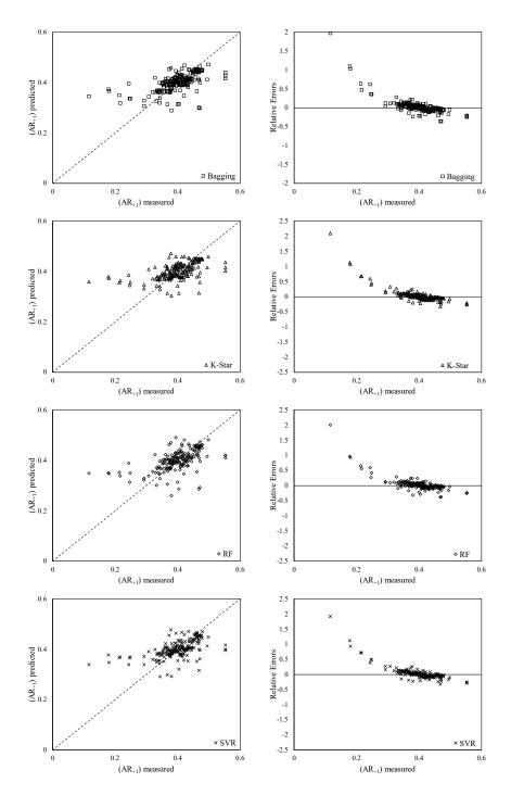
**Figure 10.** Aspect ratio prediction "Model 1": in the left column, predicted versus experimental values, in the right column, residuals versus experimental values.
