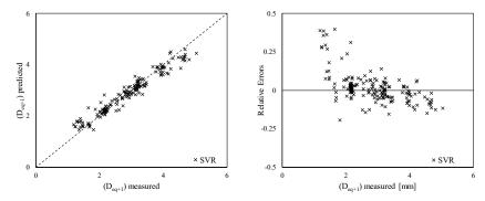
**Figure 6.** Equivalent diameter prediction "Model 1": in the left column, predicted versus experimental values, in the right column, residuals versus experimental values.
