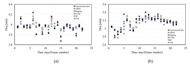
**Figure 9.** Comparison among equivalent diameters by means of time series; **(a)** Model 1—bubble 1; **(b)** Model 2—bubble 12.
