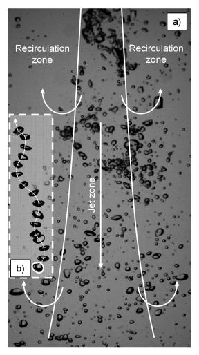
**Figure 1.** Air bubbles entrained by the vertical plunging jet (**a**); individual air bubble path, rising inside the lateral recirculation zone (only the highlighted bubble is at the same time as the recorded frame) (**b**).
