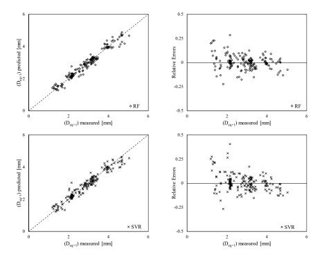
**Figure 7.** Equivalent diameter prediction "Model 2": in the left column, predicted versus experimental values, in the right column, residuals versus experimental values.
