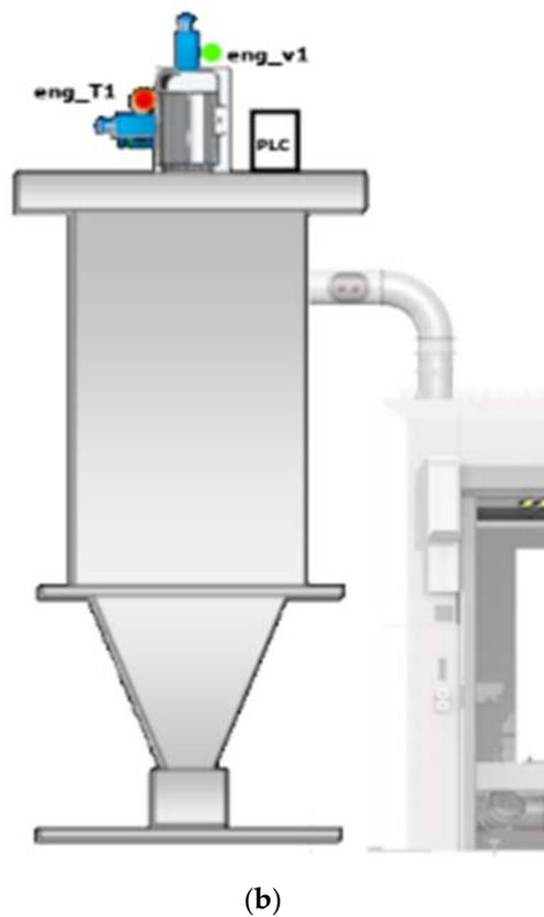
**Figure 3.** Example of a waterjet machine with the cyclone and sketch of sensors (red and green circles). (a) Waterjet machine. (b) Sensors placement sketch.
