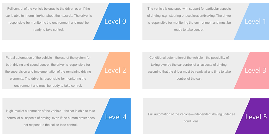
Figure 3. Autonomous driving levels—the International Society of Automotive Engineers (SAE) classification.
