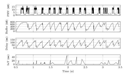
**Figure 2.** System parameters with distance and traffic rate of 30 m and 50 Mbps, respectively, using the greedy scheduler.
