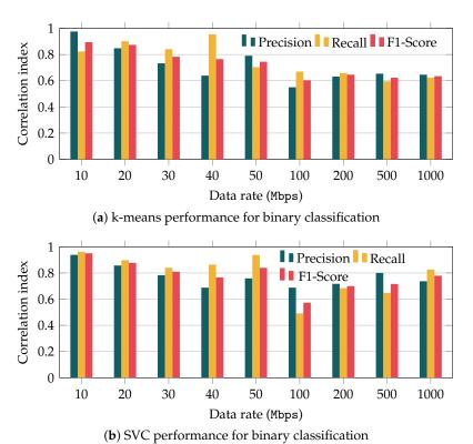
Figure 9. Performance of binary classification for a distance of 40 m and the different data rates.
