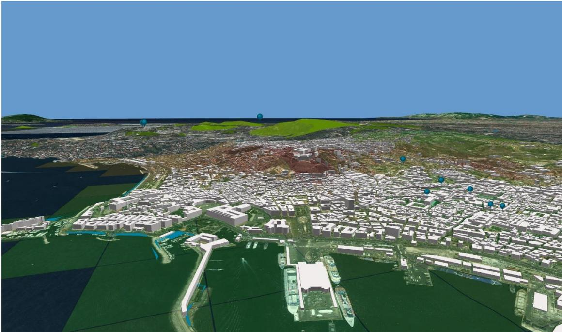
**Figure 5.** Excerpt of the 3D city model with the UES grid overlapped. The spatial relationships among building z-values and Regulation Services cell values are visualised.
