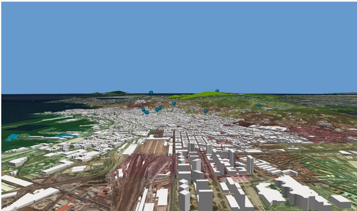
**Figure 4.** Excerpt of the 3D city model with the Urban Ecosystem Services (UES) grid overlapped. The spatial relationships among building z-values and Regulation Services cell values are visualised.
