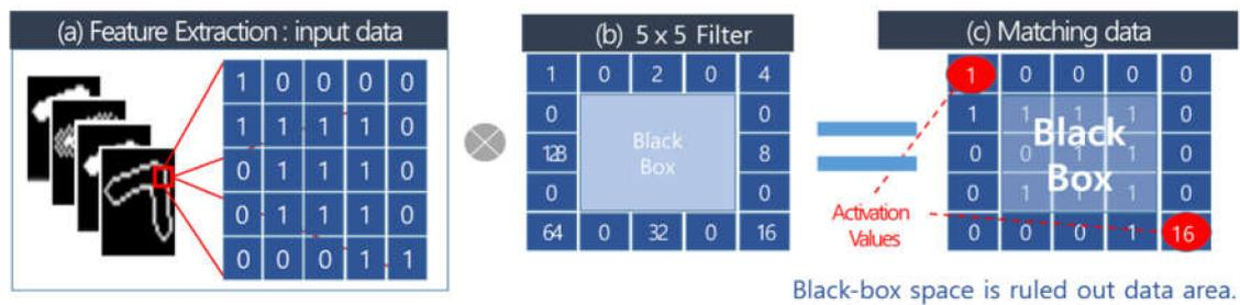
**Figure 7.** The process of activating the area extraction using the  $5 \times 5$  filter.
