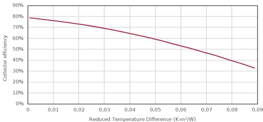
**Figure S7.** Solar thermal collector efficiency curve, as a function of the reduced temperature difference. The latter is defined as the difference between (a) the average fluid temperature between
