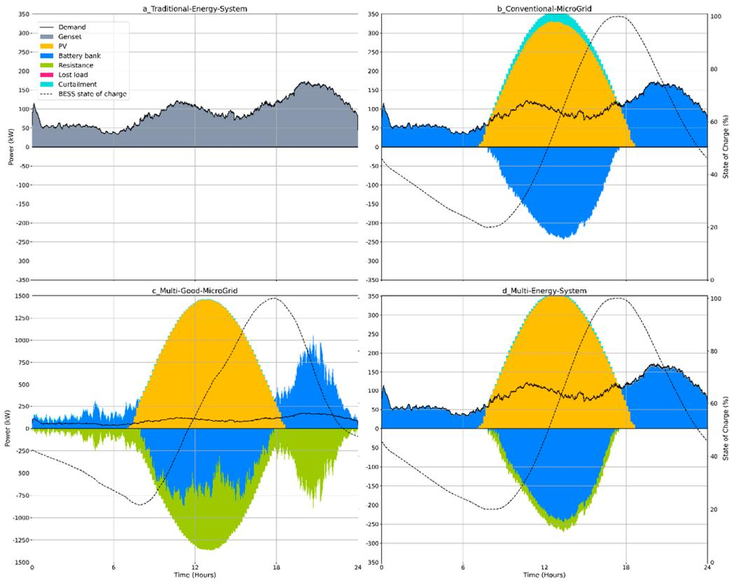
**Figure S2.** Autumn Electric energy dispatch strategy in the four modelled scenarios, namely: (a) Baseline; (b) Conventional micro-grid; (c) Multi-good micro-grid; (d) Integrated multi-energy system. The represented day is March 21st.
