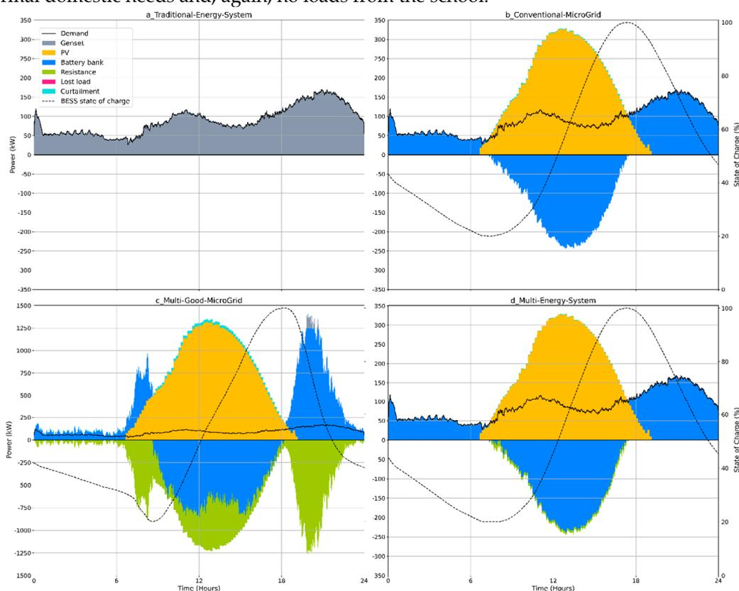
**Figure S1.** Summer Electric energy dispatch strategy in the four modelled scenarios, namely: (a) Baseline; (b) Conventional micro-grid; (c) Multi-good micro-grid; (d) Integrated multi-energy system. The represented day is December 21st.
