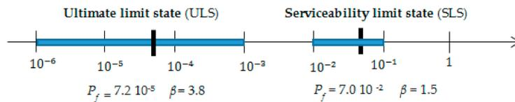
**Figure 1.** Reliability index  $\beta$  on the numerical axis for load-bearing elements of reliability class RC2.
