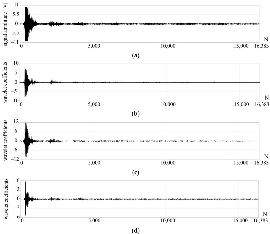
**Figure 7.** Registered signal for a plate with a recess (a), detail 1 (b), detail 2 (c), detail 3 (d) of DWT, Daubechies 8 wavelet, N—number of time intervals.
