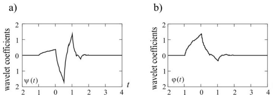
Figure 2. Daubechies 4 wavelet: (a) basis function (mother), (b) scaling function (father).
