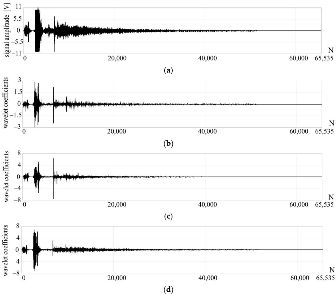
**Figure 8.** Registered signal for a plate with two apertures (a), detail 1 (b), detail 2 (c), detail 3 (d) of DWT, Daubechies 8 wavelet, N—number of time intervals
