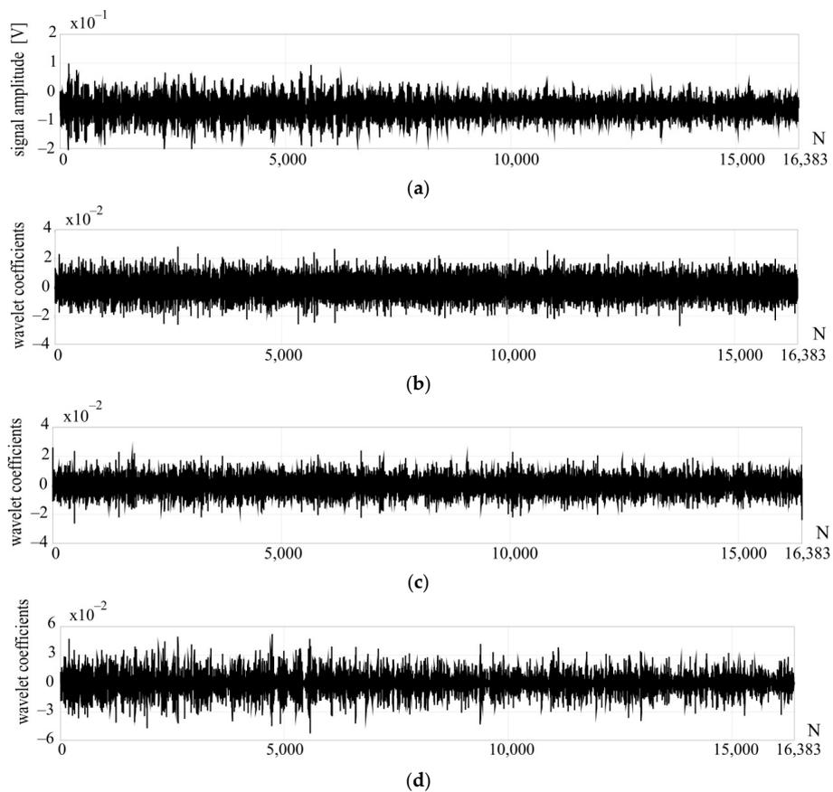
Figure 6. Registered signal for an undamaged plate (a) detail 1, (b) detail 2, (c), detail 3 (d) of the discrete wavelet transform (DWT), Daubechies 8 wavelet, N—number of time intervals.
