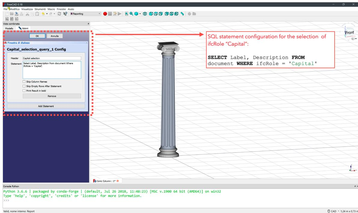
**Figure 13.** SQL query performed by using predefined statements and datasheet report in order to investigate *Capital* IFC custom role and its description: on the left side of FreeCAD is the SQL statement preparation for custom query.
