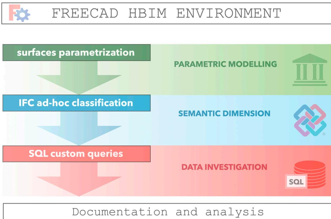
**Figure 21.** FreeCAD HBIM environment for documentation and analysis: from 3D parametric modeling based on predefined libraries and parametrization of imported surfaces; ad hoc semantic dimension through custom IFC classification and other attributes; ad hoc SQL queries for data investigation.
