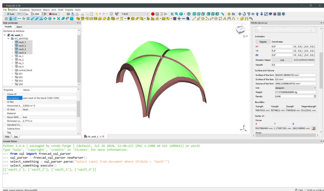
**Figure 12.** SQL query performed on Python console in order to investigate *Vault* IFC custom role: results in green text inside square brackets after the SQL query syntax.
