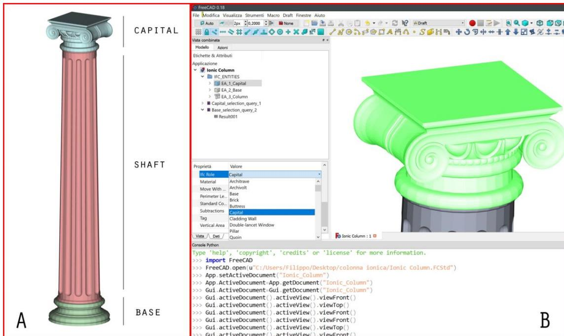
**Figure 4.** Example of ionic column. (A) Ionic column subdivisions: capital in blue; column shaft in red; base in green. (B) FreeCAD experimentation: IFC classification of the ionic capital by using custom roles available on the drop-down menu after the implementation.
