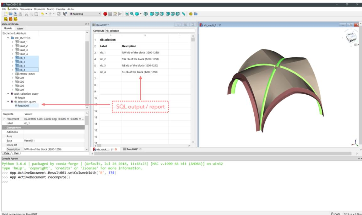
Figure 16. SQL query in order to investigate Rib IFC custom role referred to rib vault and their description: on the left side are the saved rib\_selection\_query and the related datasheet report with the query result.
