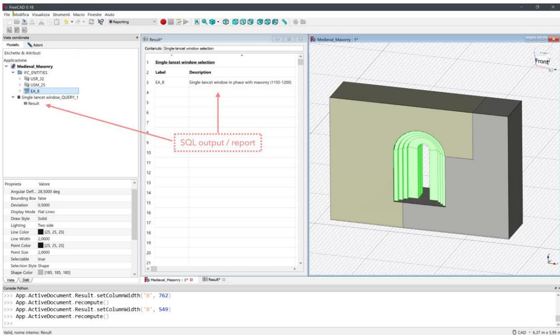
Figure 18. SQL query in order to investigate *single-lancet window* IFC custom role and its description, referring to the medieval wall: on the left side are the saved *single-lancet window\_query\_1* and the related datasheet report with the query result.
