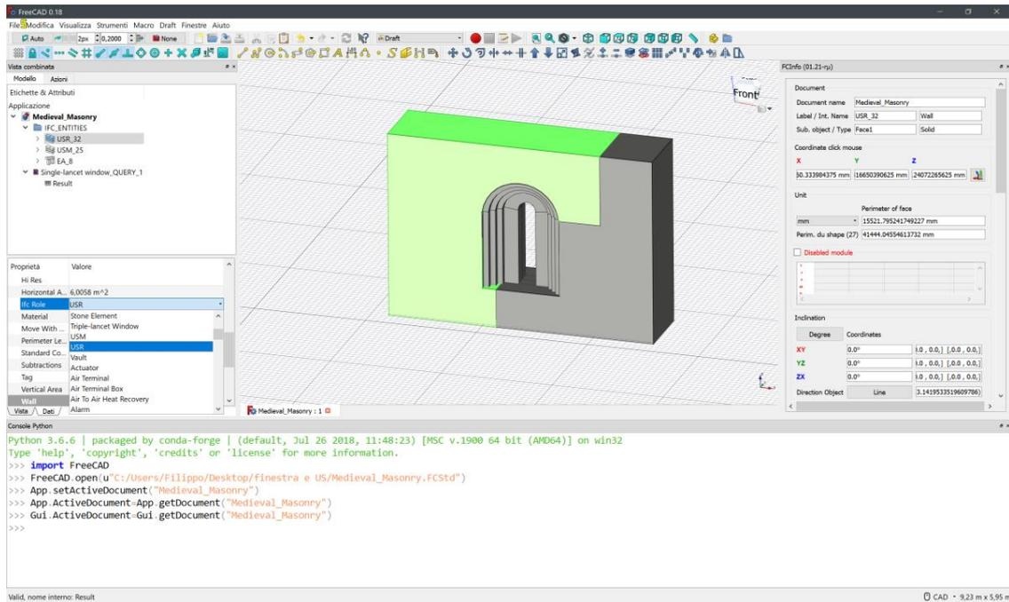
**Figure 10.** Example of a medieval stone wall: IFC classification of plaster layer on masonry as render stratigraphic unit (USR on the left of single-lancet window—see also Figure 7) available on the drop-down menu after the implementation of ifcWall entity and ArchComponent.py.
