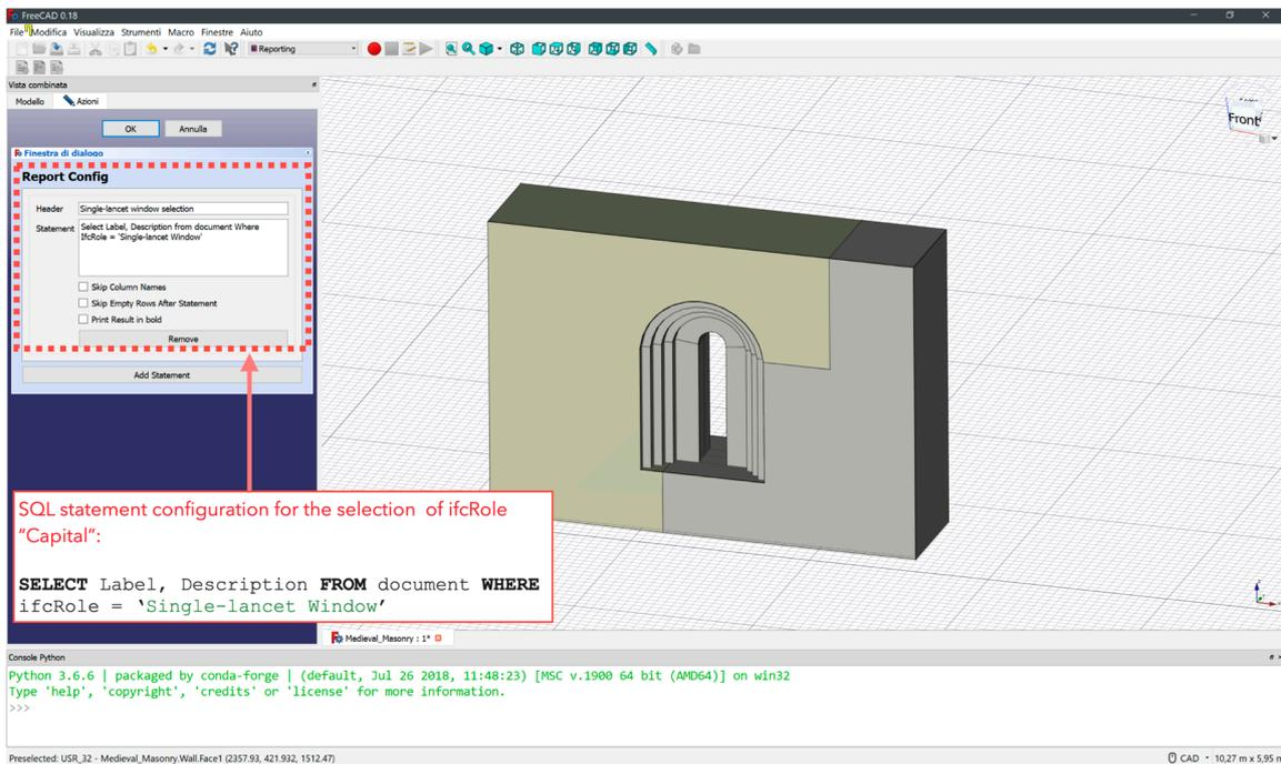
Figure 17. SQL query performed by using predefined statements and datasheet report in order to investigate *single-lancet window* IFC custom role and its description: on the left side is the statement preparation.
