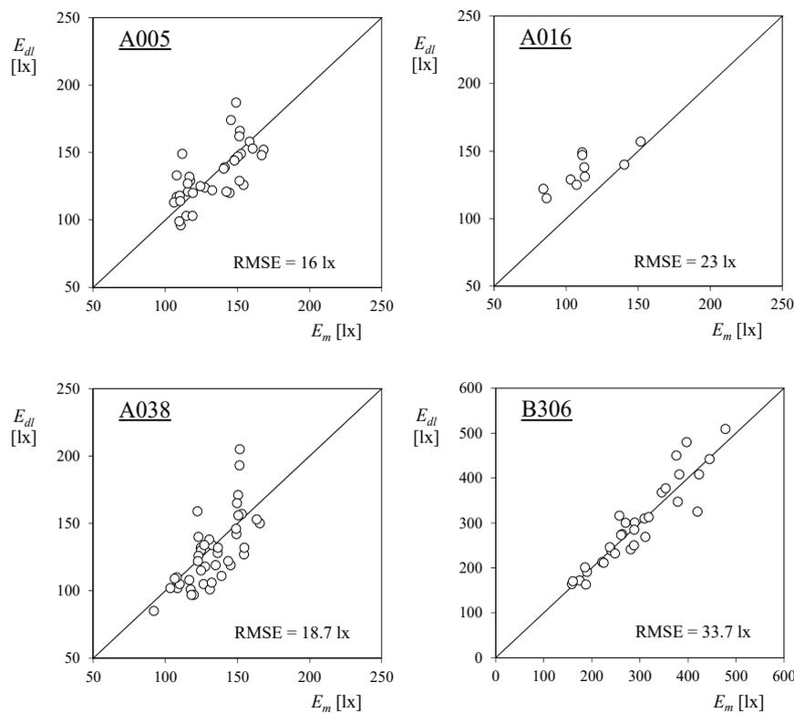
**Figure 8.** Illuminances calculated by DIALux®,  $E_{dl}$ , on each of the desks in classrooms A-005, A-016, A-038, and B-306, compared to the measurements taken in each case,  $E_m$ : A line indicating the ideal simulation is included on each graph. The Root Mean Square Error (RMSE) of  $E_{dl}$  in relation to  $E_m$  is included in each graph.
