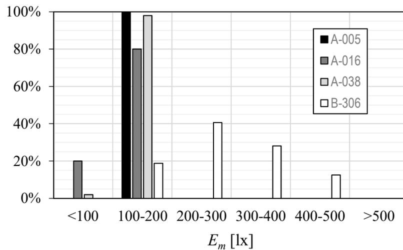
**Figure 7.** Percentage distribution of the individual desks with regard to the measured illuminance,  $E_m$ , in the classrooms selected for this study (A-005, A-016, A-038, and B-306).
