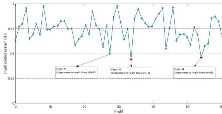
Figure 7. The CHI of flight control system.
