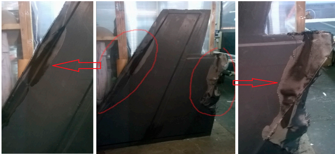
Figure 8. The non-impregnated edges of the cured tail panel in its corners ( right ) and on the periphery ( left ). The full view of the ready defective part is shown in the center photo.
