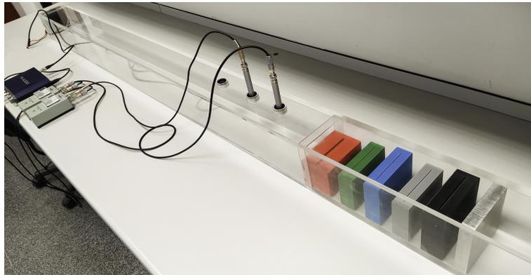
**Figure 3.** Experimental setup used to measure the reflection and absorption coefficients in an impedance tube for a 1D system of Helmholtz resonators. The impedance tube includes a loudspeaker controlled by a sound card at one end and the set of Helmholtz resonators at the other end, backed by a rigid surface. Two microphones are mounted on the tube walls as specified in reference [45].
