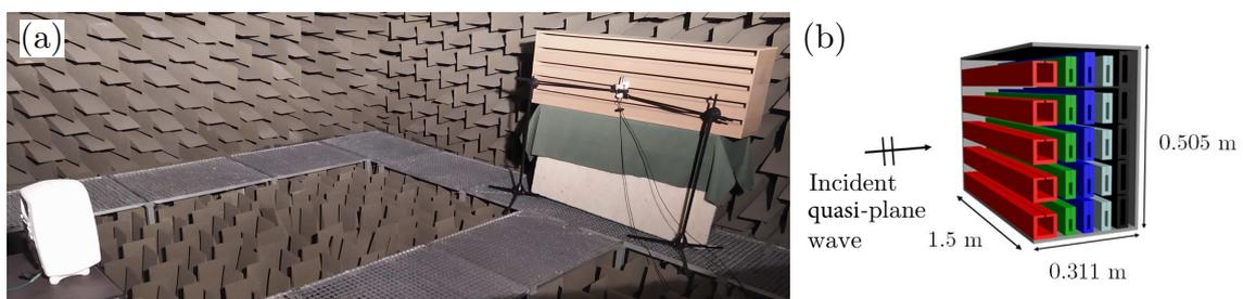
**Figure 4.** Experimental setup of the 2D finite array of Helmholtz resonators inside the anechoic chamber. (a) Picture of the experimental configuration. (b) Schematic diagram of the 2D system of Helmholtz resonators.
