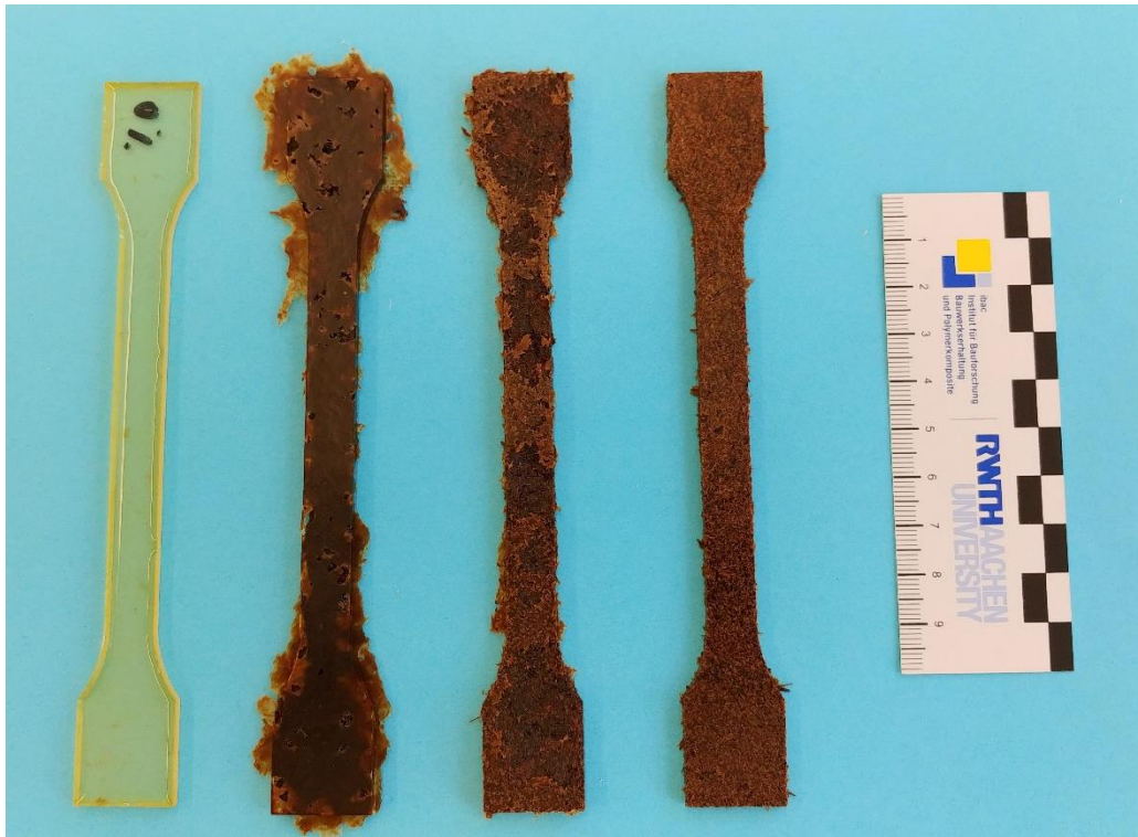
Figure S5. Optical appearance of the Gg1-1 specimen with increasing feather content. From left to right: 0 (Gg1-1), 5, 10, and 20 wt% (Gg1-1F). The first and the last sample are taken from a series that was used to assess the tensile properties (cf. Tab. F and Figs P, S6, S7).
