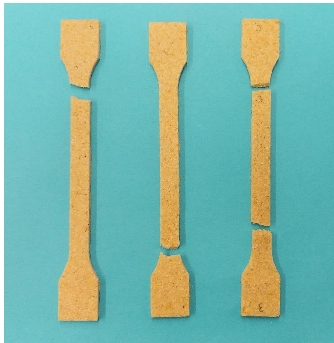
Figure S6. The 3 Cg1-1F samples after tensile testing.
