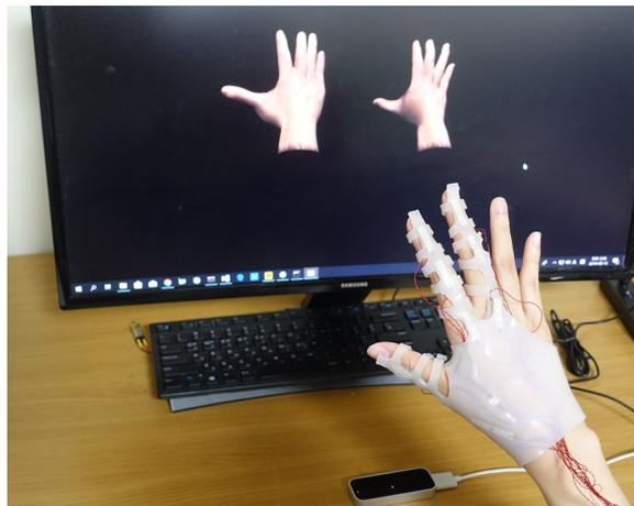
**Figure 3.** Interface for generating virtual hand using sensor data and leap motion sensors. The virtual hand in the left of the screen is generated through processing of piezoelectric sensor data and the hand on right of the screen is directly related to leap motion sensor.
