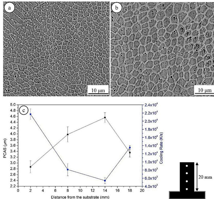
**Figure 6.** SEM images of DED AISI 316L at: (a) 2 mm, (b) 14 mm from the deposition/substrate interface, (c) primary cellular arm spacing (PCAS) and cooling rate as a function of the distance from the substrate [37].
