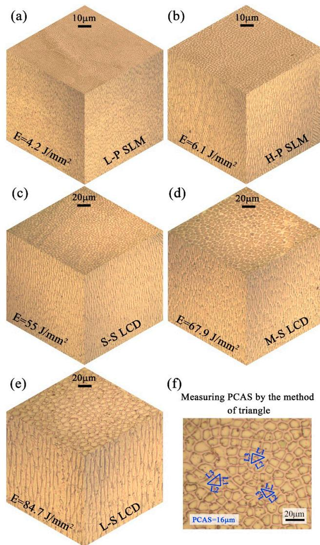
**Figure 7.** 3D composite view showing the cellular morphologies of the five kinds of typical samples at the processing parameters of (a) low-power laser powder bed fusion (LPBF), (b) high-power LPBF, (c) small-size DED, (d) middle-size DED, and (e) large-size DED. (f) Schematic sketch of measuring PCAS by the three-angle method [49].
