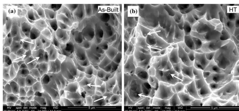
**Figure 15.** Fracture surfaces of AISI 316L stainless steel: (a) as-built and (b) heat-treated. Arrows mark a few of the many examples of fine particles observed resting inside ductile dimples throughout the fracture surface [90].
