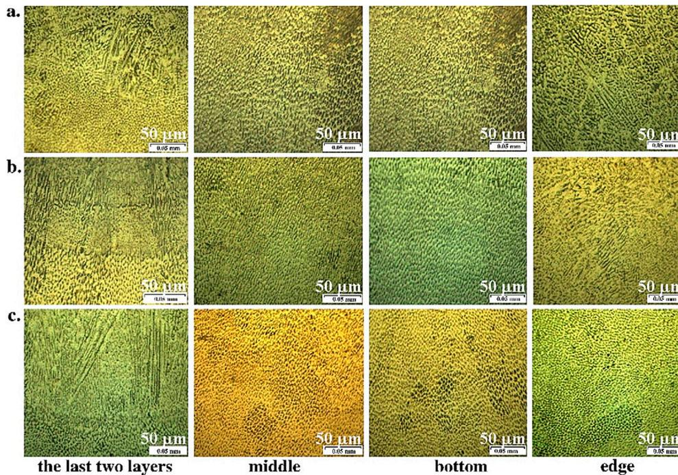
**Figure 5.** The microstructure of the DED thin walls examined at cross-section and longitudinal section in the middle of the thin wall. (a) With a constant laser power of 300 W, (b) Process control with a constant set-value 0.5 V and (c) Process control with a path-dependent set-value 0.3 V (2 mm)–0.5 V (56 mm)–0.3 V (2 mm) [52].
