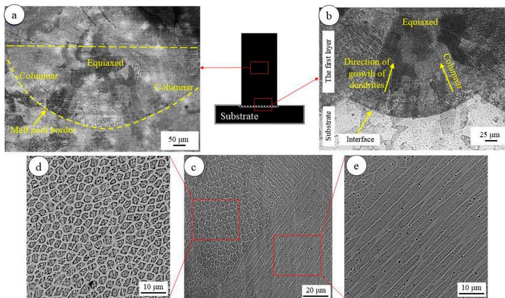
**Figure 4.** Light optical microscopy micrographs of the DED AISI 316L steel samples produced by DED: (a) a representative melt pool at the middle height, (b) the microstructure of the first layer, (c) SEM images of the columnar and equiaxed microstructures referring to the last deposited layer, (d,e) high magnifications of (c) from two different regions [37].
