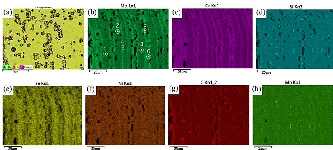
**Figure 11.** Element mapping for deposition body area: (a) layered element image, (b) molybdenum and target body, boundary element composition points, (c) chromium, (d) silicon, (e) iron, (f) nickel, (g) carbon, (h) manganese [41].
