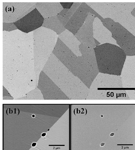
**Figure 12.** Oxide inclusions in the fully-recrystallized additive manufacturing (AM) AISI 316L stainless steel: (a) low magnification back-scattered electron image; (b1) high magnification back-scattered electron image; (b2) high magnification secondary electron image [75].
