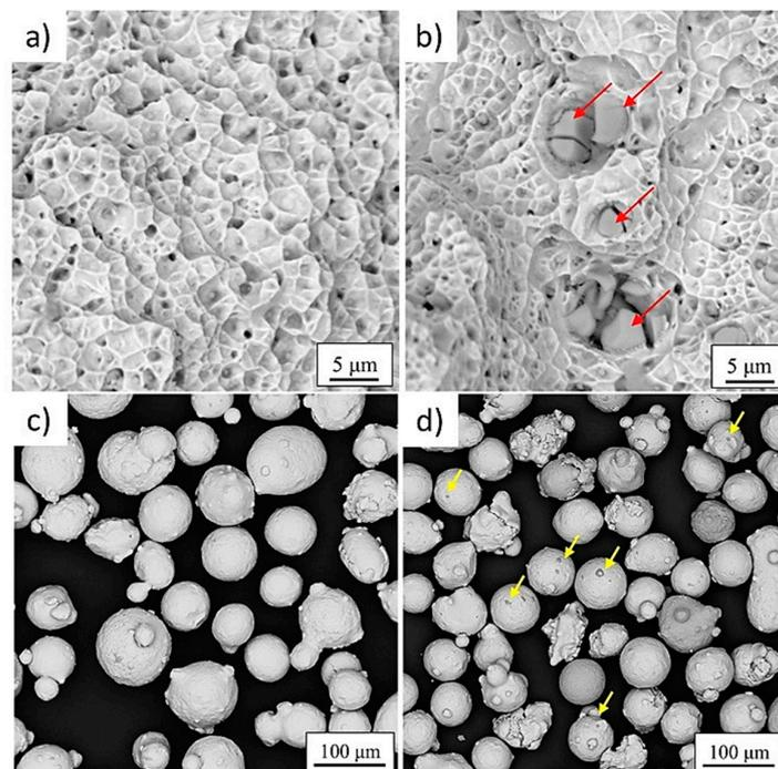
**Figure 14.** A summary of the tensile fracture morphologies of AISI 316L stainless steel samples produced by DED using (a) fresh powder and (b) recycled powder. SEM images of (c) fresh and (d) recycled AISI 316L powders [37].
