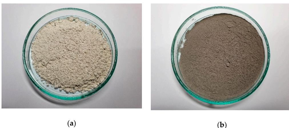
**Figure 2.** Waste-glass powder (a) and fly ash (b) used for producing the tested mixes.
