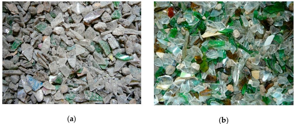
**Figure 1.** View of waste glass; raw (a) and precleaned (b).
