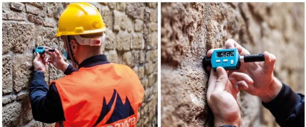
**Figure 3.** Non-destructive in situ survey with Equotip hardness tester on a masonry face of a building.
